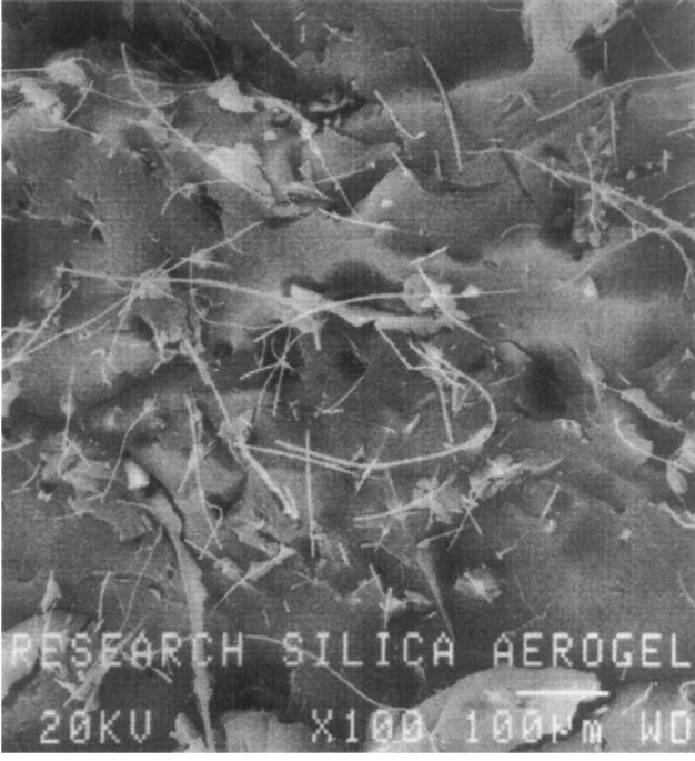
Fig. 4 SEMs of fiber-filled aerogel; magnification = 100X.
